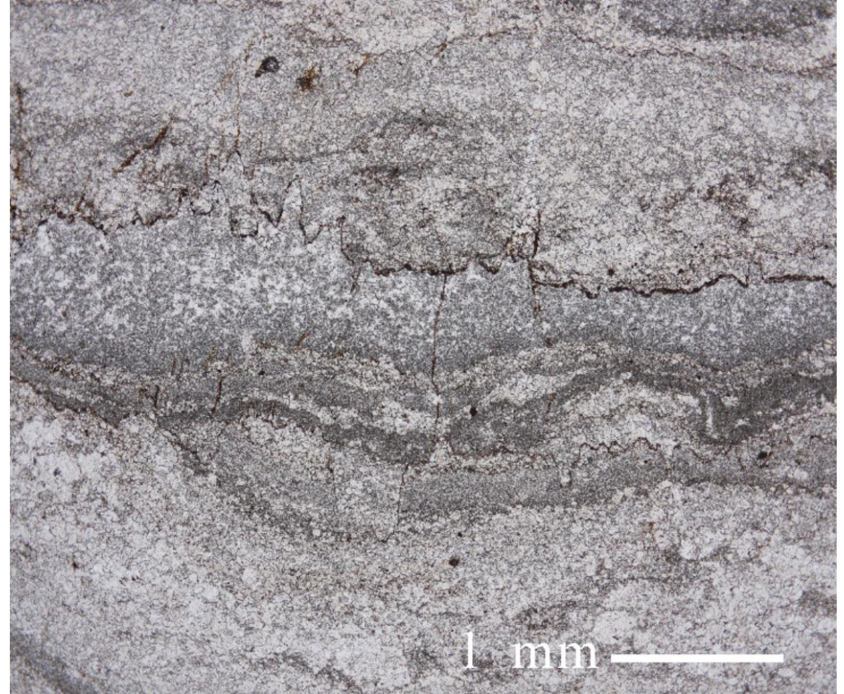
A dolomitic laminite consisting of dark micritic minilaminae and thick thrombotic laminae, from the Lower Cambrian Stage 3 in Aksu, Xinjiang, China. The sample no. is S-17.
